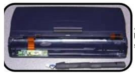
And unplug the small connector to remove the battery completely. This plug can sometimes have some sealer on it - just remove this first.
