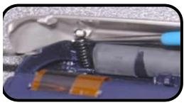
Use the spring hook or similar to remove the top loop of the spring from the small plastic hook in the rear casing. Leave the bottom of the spring attached to the bottom casing. Repeat for the other side.
