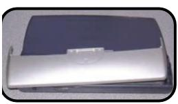
Now slide the top cover sideways (away from the pin you removed) as shown. This should release the other hinge pin.....
